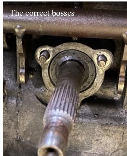
The drilled and tapped bosses with sleeve—all done in situ . (Blue paint is to show witness marks from starter ring for die-grinding—a tight fit)
