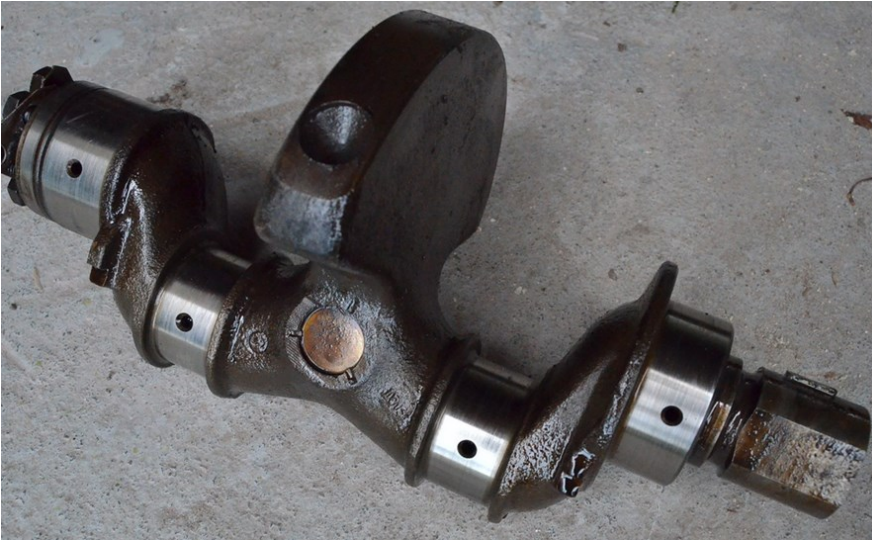
Factory crankshaft was designed for a 4700 red line, suffers from whipping at 6000 rpm and likely catastrophic failure if sustained above that.
