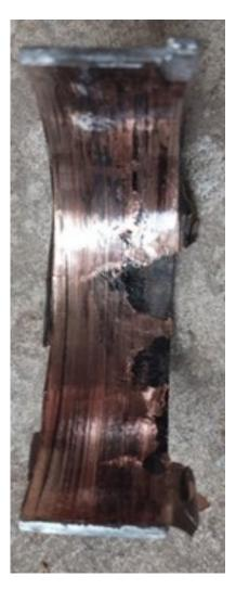
lack of power down the straight. Aware something was off, I pulled into the pits. While going down the pitlane, I could hear a very subtle, yet unmistakable death rattle associated with big end bearing failure. I dreaded the thought of another big end bearing going. To put my mind at ease, and confirm what the rattle was, I ripped the sump off, unbolted big end cap #1. There it was, one destroyed big end bearing-my race was over. I spent the remainder of the event on a flag point.
