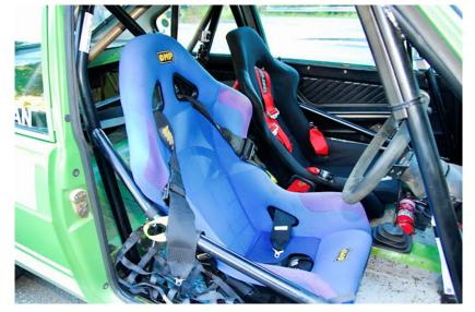
Considering how long the gear shift is, cog-swapping was remarkably precise but not superrapid. The standard pattern fivespeed relies on a solid rod from the shifter to the 'box itself, which is mounted behind the engine in what's a quite rare and very Alfa—north / south, front wheel drive configuration.
