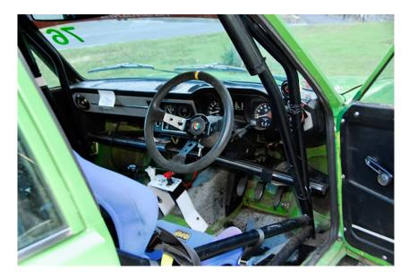
and rear. The ride was firm with no discernible body roll, or pitching under deceleration. The entire chassis was impressively rigid, which is no doubt aided by the inclusion of the aforementioned Targa-spec roll cage.
