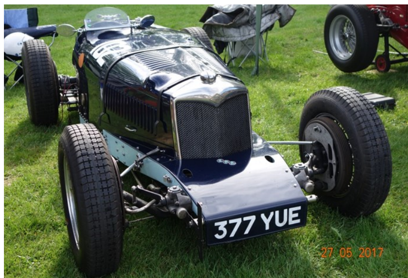
1933 Riley (rare ERA prototype) – supercharged 2 litre 6 cylinder that can reach 100km/h in 4 sec.
